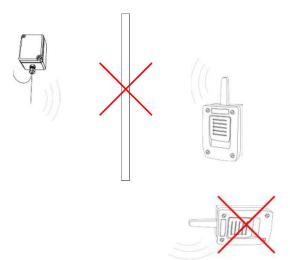
The transmitter and receiver antenna must be parallel to each other for optimum signal reception
