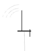
868MHz AED-868 or FLAT 868 antenna extension with RG 58 coaxial cable
