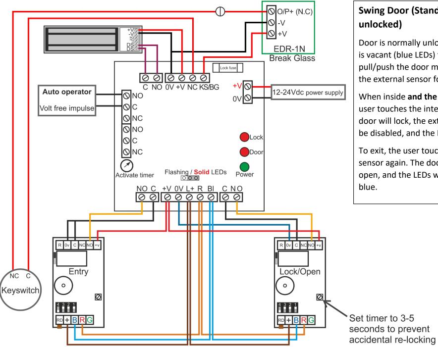
Door is normally unlocked. If the facility is vacant (blue LEDs) the user can pull/push the door manually or touch the external sensor for assisted entry.
