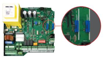
Fixed 12 Vdc output for an electric lock up to 3A
