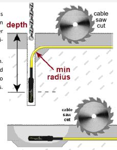
When setting the lead in black top, use a packer or sand layer as protection against hot pitch sealing. Setting in a sand course below **paving** is ideal. Poly-pipe is also recommended for fitting in gravel.
