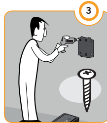
DRILL HOLES IN THE WALL
