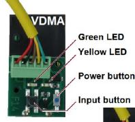
VD964a connections Only yellow LED works with VD964a. Green does not.
