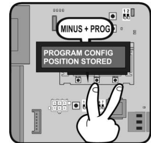
PRESS MINUS + PROG TO STORE CLOSING POSITION
