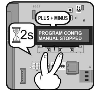
PRESS MINUS + PROG TO STORE CLOSING POSITION
