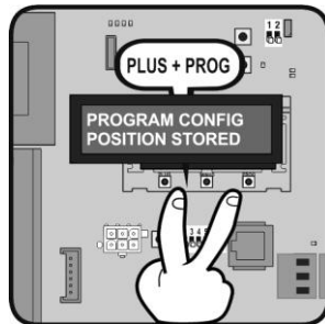
PRESS PLUS + PROG TO STORE OPENING POSITION
