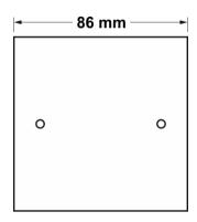
Attach the plate to box using the two 3.5mm screws supplied
