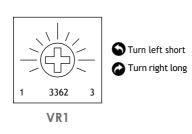
The activation switch is default with Time delay. Adjustable range 0.3-30s.
