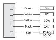
A permanent supply is required to operate the touchless activation switch to provide all functions.
