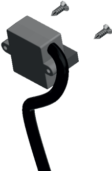
Closing of the protective enclosure
