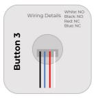
Instead of using the 2 blue wires, you are using red & blue for NO.
