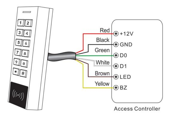
When set to reader mode, brown and yellow wires are redefined to green LED control and buzzer control respectively.
