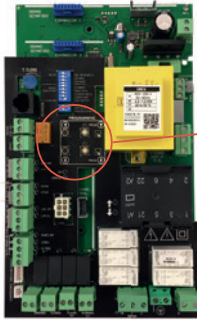
Easy to program Programming buttons on the board
