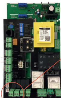
Lock function Door open and door closed signal
