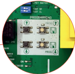
Easy to program Programming buttons on the board
