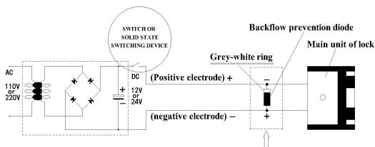
Connection method of backflow prevention diode:
