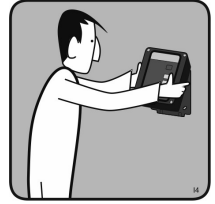
HANG CONTROL PANEL
