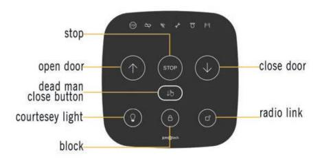
Turn on dipswitch 1 and press and hold the open & close buttons to check the door runs in the correct direction. If not, press the courtesy light (bulb) button to change it.
