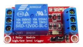
These units function as both a Lowlevel trigger or High level trigger by using the jumper or insert link & use as conventional relay.
