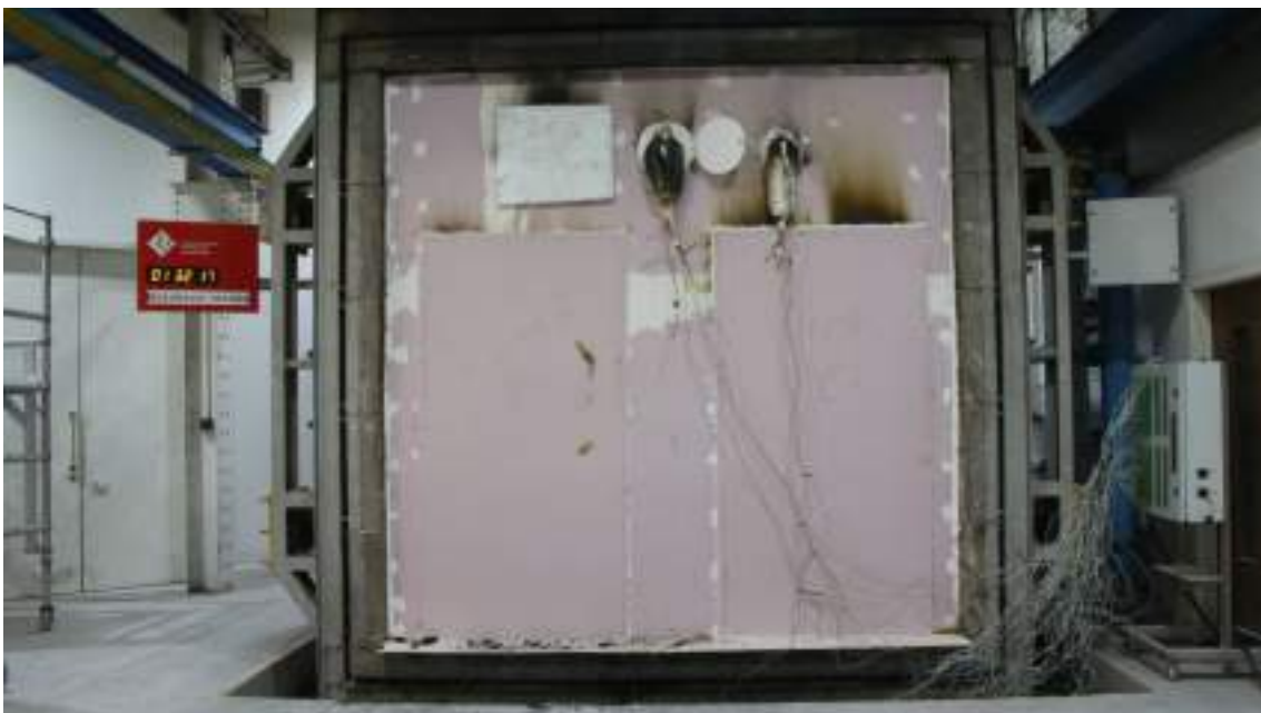
Figure 26 - The unexposed surface of the test construction after a test duration of 92 minutes
