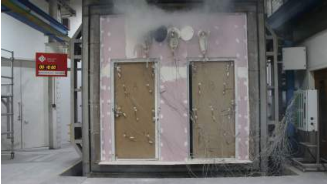
Figure 19 - The unexposed surface of the test construction after a test duration of 10 minutes
