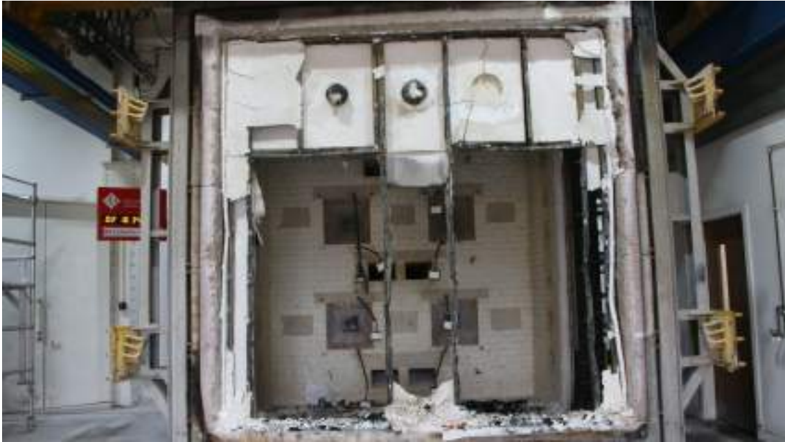
Figure 33 - The exposed surface of the test construction after the test was discontinued
