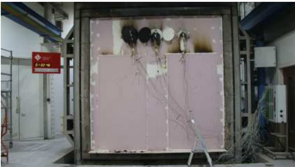
Figure 24 - The unexposed surface of the test construction after a test duration of 62 minutes
