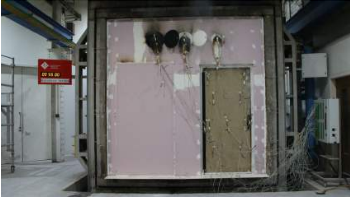
Figure 23 - The unexposed surface of the test construction after a test duration of 55 minutes
