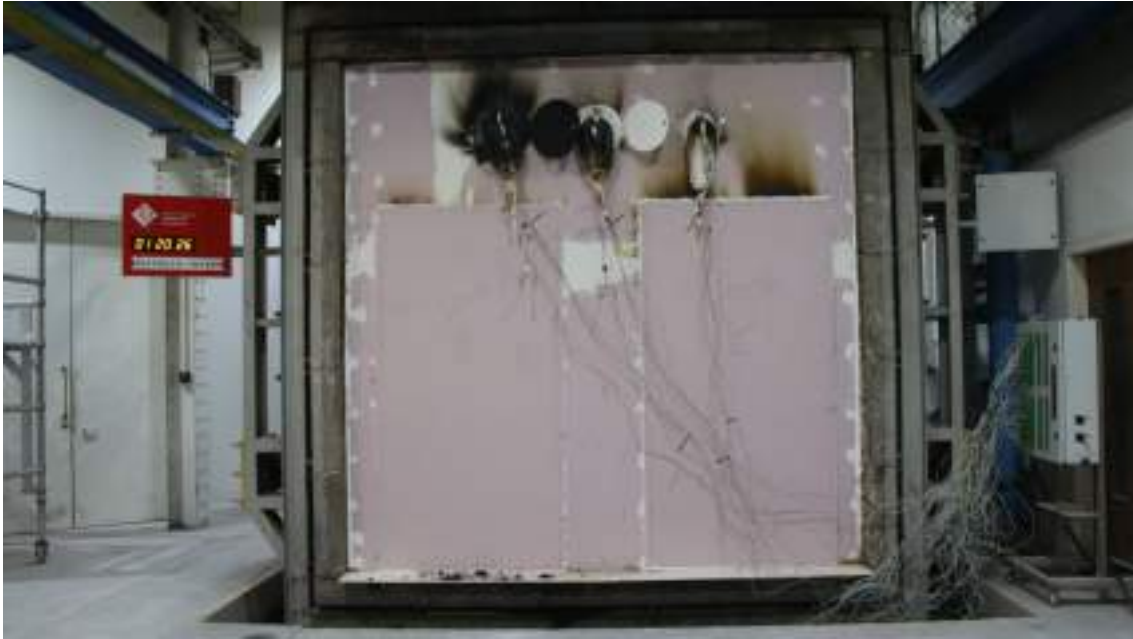
Figure 25 - The unexposed surface of the test construction after a test duration of 80 minutes
