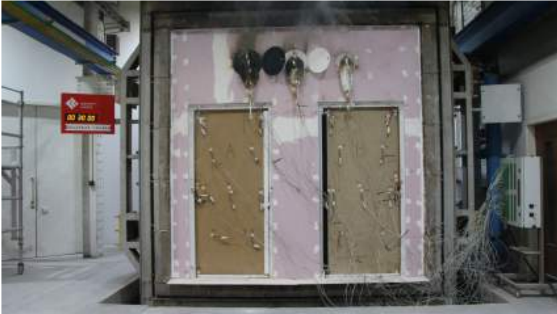
Figure 21 - The unexposed surface of the test construction after a test duration of 30 minutes
