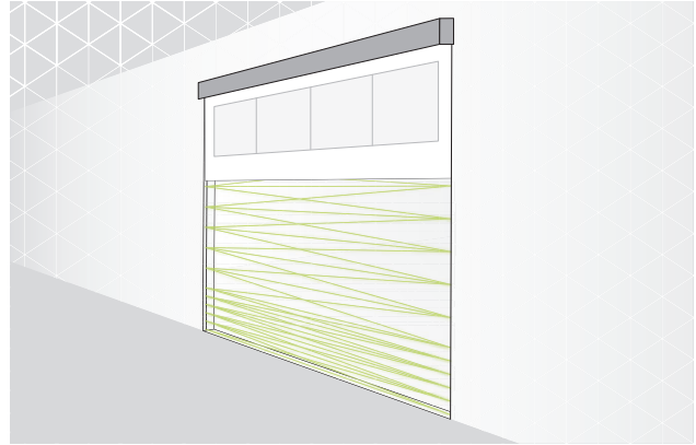
Figure 4: High-speed doors with door blanking
